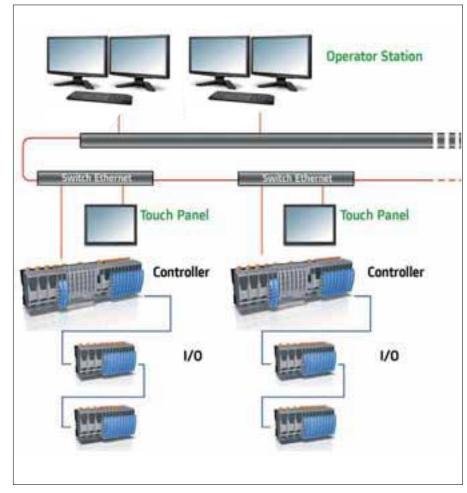
It features a I/O slice system for the highest granularity, offering a minimal number of channels per module for most economic solutions.
