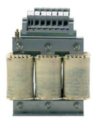
In connection with the mains chokes, converters and infeed power supply units realize higher DC bus continuous power. They reduce the harmonics in the line current while simultaneously preventing troublesome mains feedback. When using supply units with line regeneration, these components are always required. This combination always complies with the permissible EMC values for industrial networks stipulated by EN 61000-2-4.
