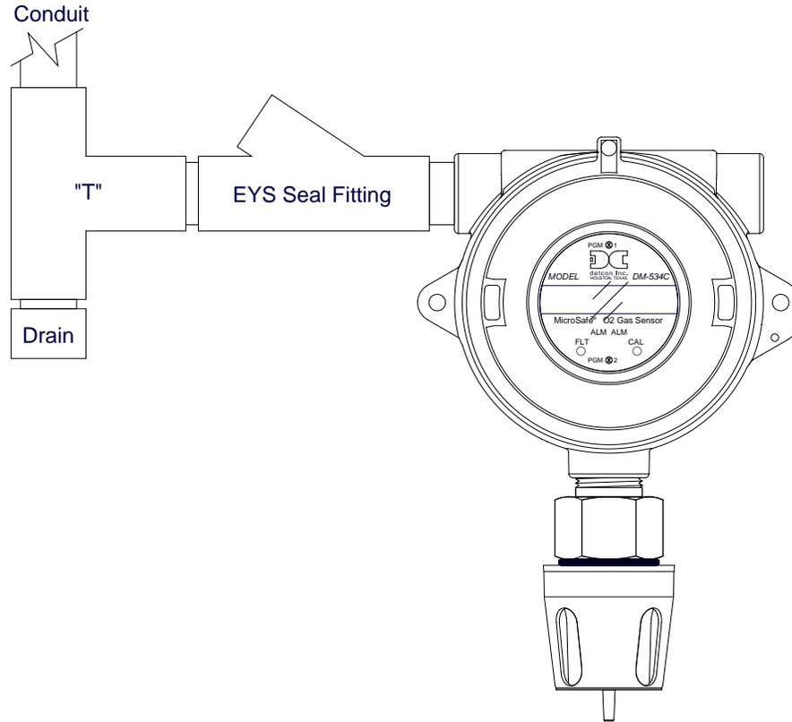
Figure 6 Typical Installation
