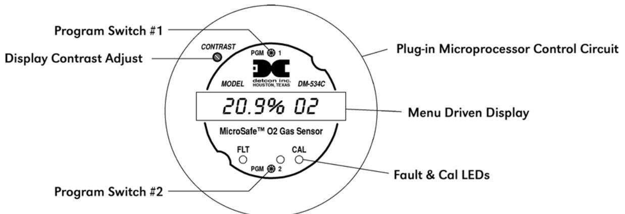
**Figure 2** Microprocessor Control Circuit
