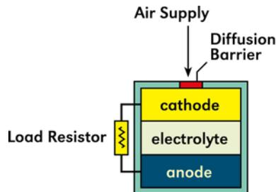
**Figure 1** Construction of Galvanic Cell
