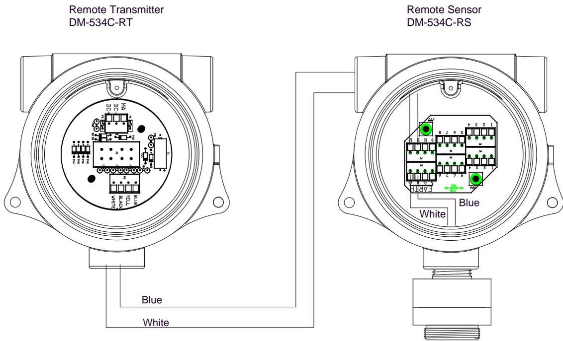
Figure 9 Remote mounting application
