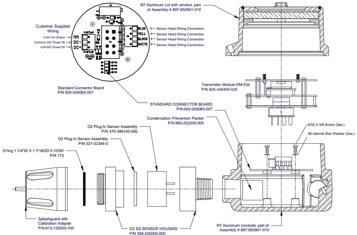
**Figure 11** Spare parts diagram
